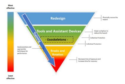
An exoskeleton can be considered a piece of work equipment. Therefore, it is a second-level measure that should not replace the implementation of technical measures at the source. An exoskeleton is a palliative solution that does not eliminate the hazard.
